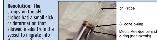
Figure 3. Internal pH probe with media leaking past o-ring.
