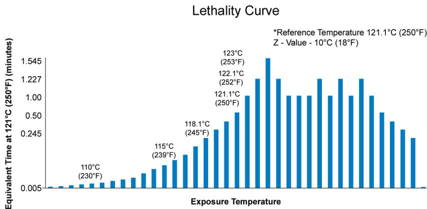
Figure 8.  $F_0$  as a function of temperature.
