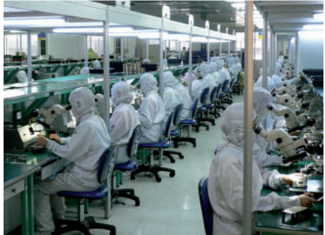
Workers assemble and test fiber optic systems. Photo: Steve Jurvetson / Wikimedia Commons / CC-BY-2.0
