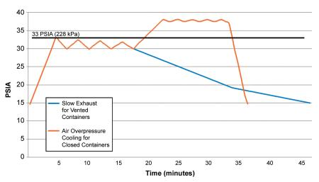
Figure 3. Typical liquid cycle chamber pressure at 121°C (250°F).
