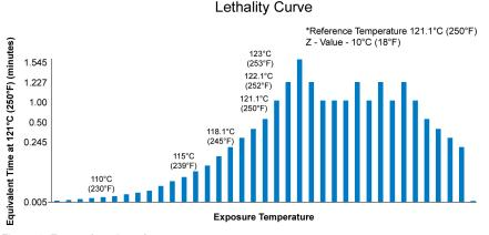
Figure 8.  $F_0$  as a function of temperature.
