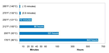
Figure 2. Sterilization time versus temperature.
