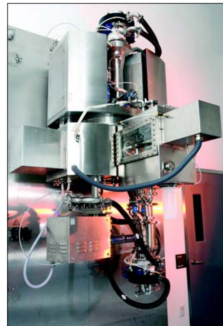
Isolated single pot process with dryer and isolated automated sampler.
